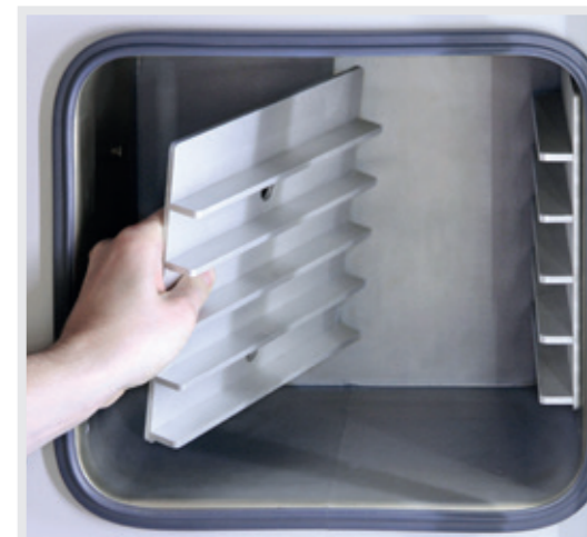
Simply removable inner sides of the chamber
