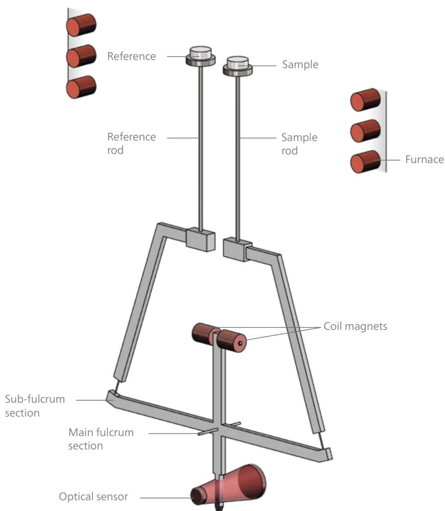
Schematic design of the top-loading differential balance of the STA 2500 *Regulus*
