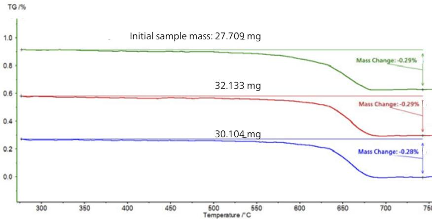
Three rubber samples from the same batch after changing the atmosphere from nitrogen to air. Heating rate 20 K/min, Pt crucibles
