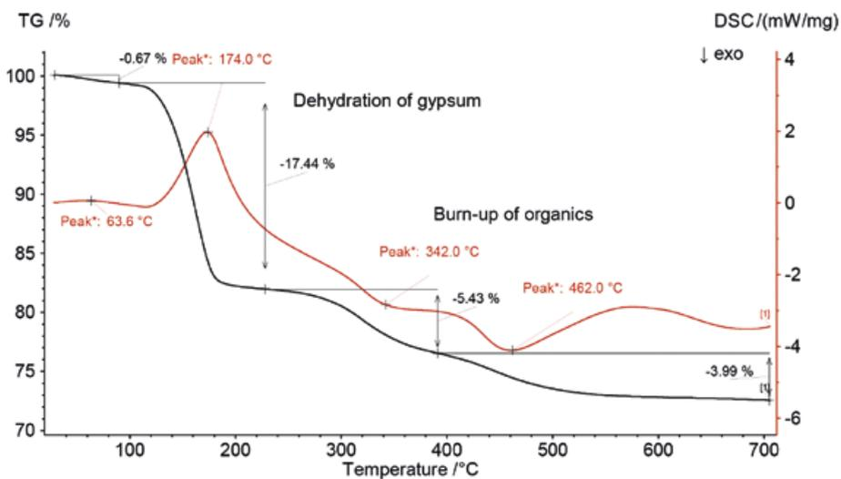
STA measurement on an aged gypsum board (8.32 mg) in air atmosphere (80 ml/min) at a heating rate of 40 K/min in open alumina crucibles. Here, the DTA signal is converted in mW/mg (DSC).
